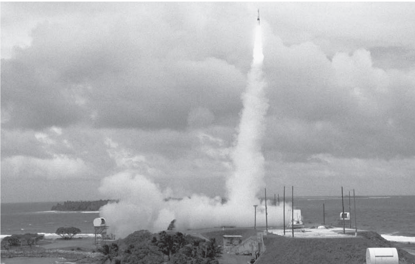
An interceptor missile is launched from the Marshall Islands December 2001 in what would prove a successful test of its ability to intercept an ICBM target, in this case a modified Minuteman ICBM launched from California's Vandenberg Air Force Base. The anti-ballistic missile system, which is currently being deployed in Alaska and California, has an inherent anti-satellite capability.
