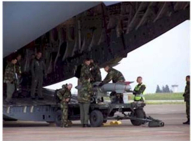
*B61 nuclear bomb, the type deployed in NATO countries, being loaded onto a C-17 cargo aircraft
